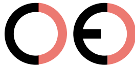
False CE Mark (too far)
